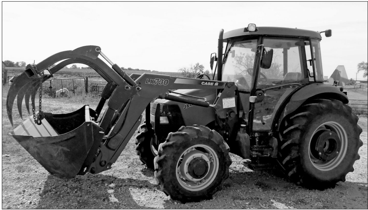
PHOTO: RITA BRHEL This 2-year-old tractor features the exterior mirrors, large window panes and downward-sloping hood that have improved operator visibility since the 1980s.
