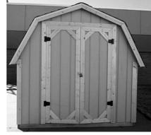
(2) 8'x12' student-built storage sheds. 2"x4" walls, 16" OC; 2"x4" treated floor joist w/3/4" cdx plywood; 2"x4" roof joists 16" OC w/30 yr. Landmark shingles. Built during the 2014-2015 school year by Yankton High School Intro to Building Trades Class.
