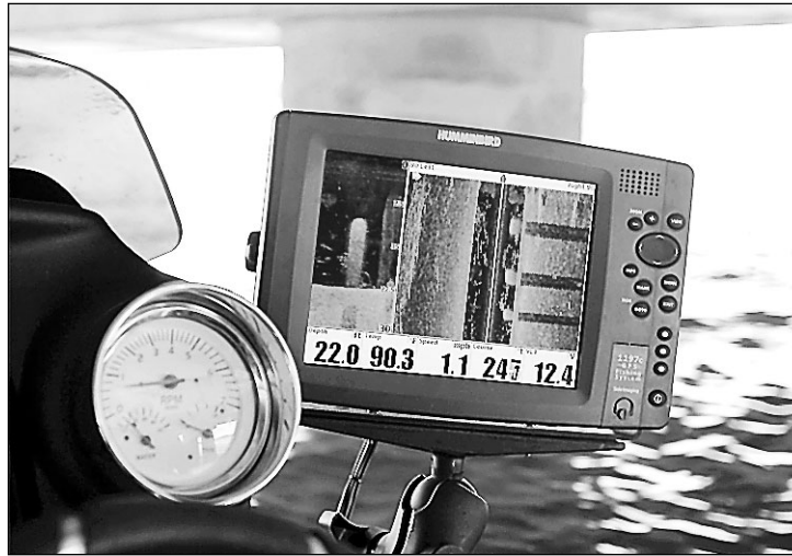
Side imaging sonar under a highway bridge distinctly shows pilings and fish near the pilings.
