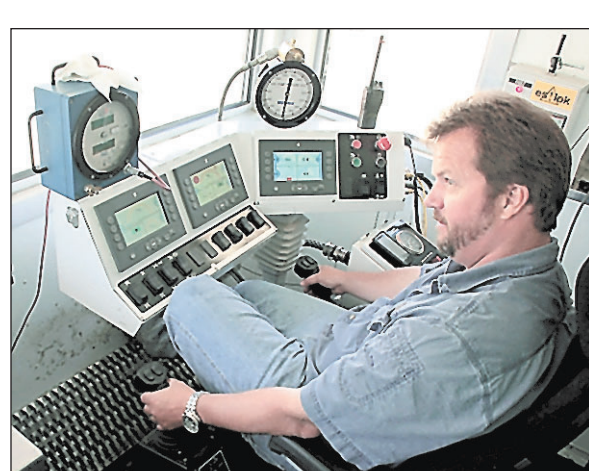
LEFT: Late last week, employees of Central Trenching, Inc. (CTI) of Minot, N.D., were working to "land" an approximately 1,500-foot directional bore under the Missouri River in this small pad of concrete just east of the Discovery Bridge on the South Dakota shore. ABOVE: Curt Curtis, a 30-year veteran of the industry, operates the directional drilling rig located just south of the Missouri River below Highway 81.
