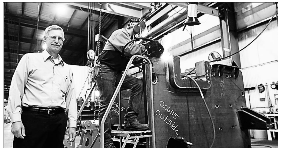
Mark Luchtel, manufacturing manager of Kolberg-Pioneer, Inc. (KPI-JCI), stands next to welder Scott VanBuren as he welds the saddle blocks on a jaw crusher base weldment in the factory in Yankton.
