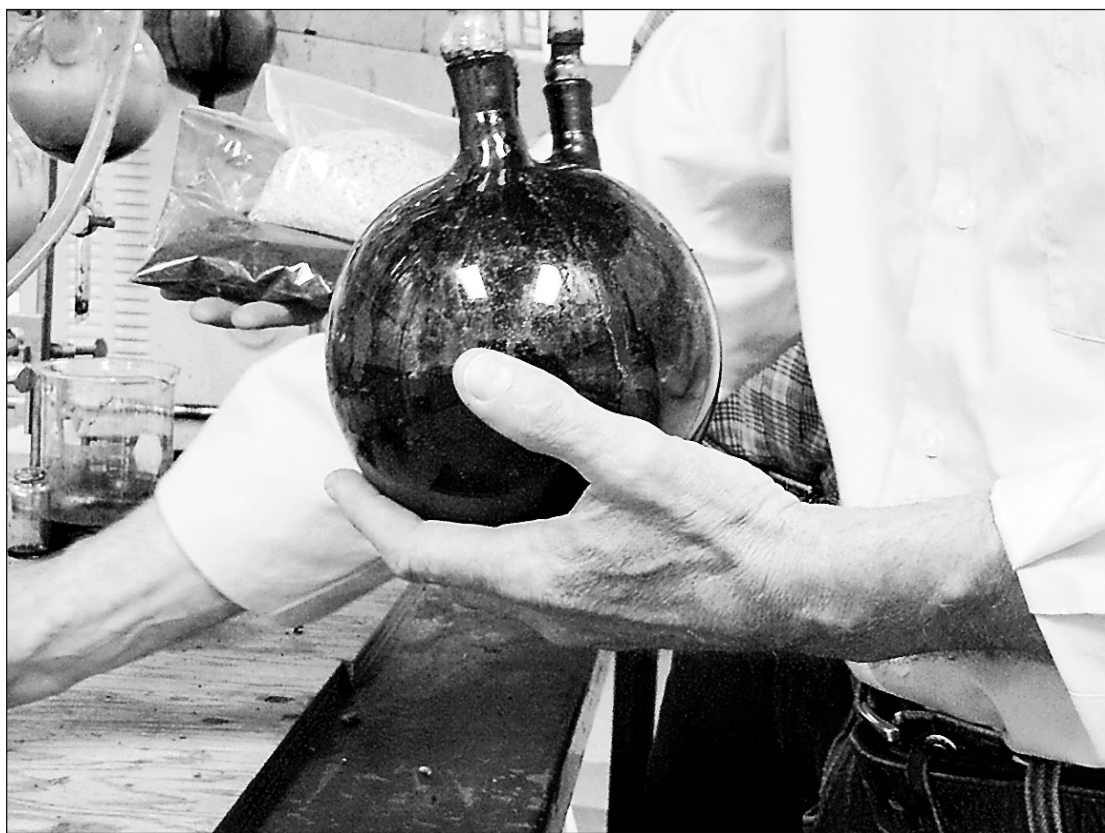
South Dakota State University scientists are researching bio-oil and a co-product called biochar. Both are produced along with a product called syngas in a process called pyrolysis.
