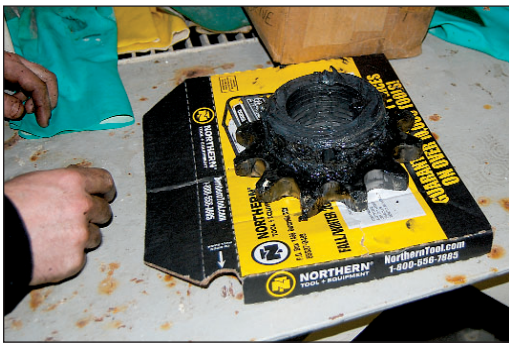
This gear on the main scraper drive in Water Plant No. 2 broke last week and cut the facility's production capacity in half. NATHAN JOHNSON/P&D
